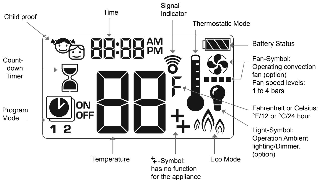
**Display hand-held transmitter including operation ambient lighting and/or convection fan (option)**
