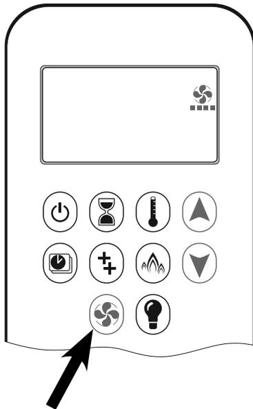
The convection fan turns automatically ON and OFF and has 4 rotational speeds which can be adjusted from low (1 bar) to high (4 bars).
