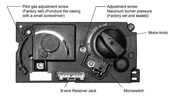
Figure 4: Gas regulating block
