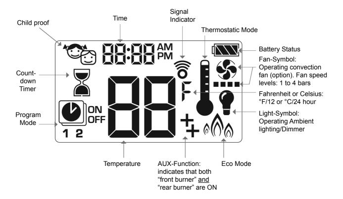
Figure 2: Display hand-held transmitter
