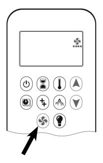
The convection fan turns automatically ON and OFF and has 4 rotational speeds which can be adjusted from low (1 bar) to high (4 bars).
