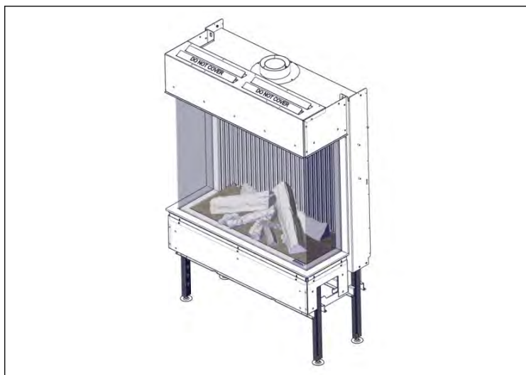
Figure 24. Aligning with adjustable height legs
