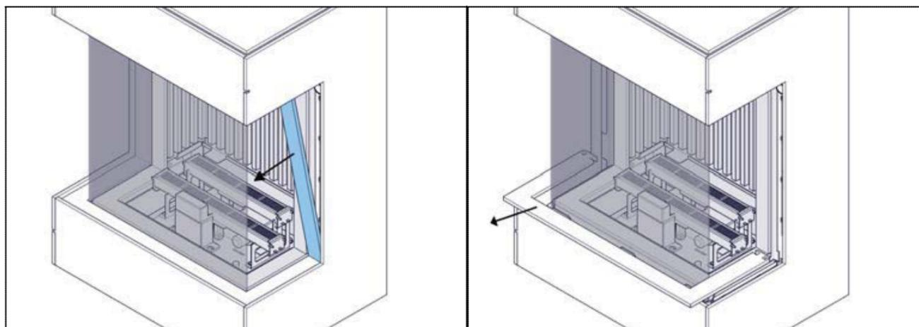
3. Unlock the fastening levers on the top left and right of the glass panes.
