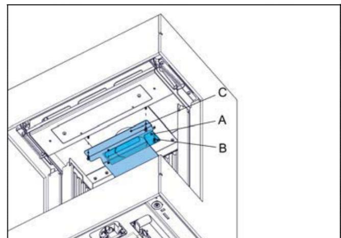
**4.2.10 Remove the baffle plate**
