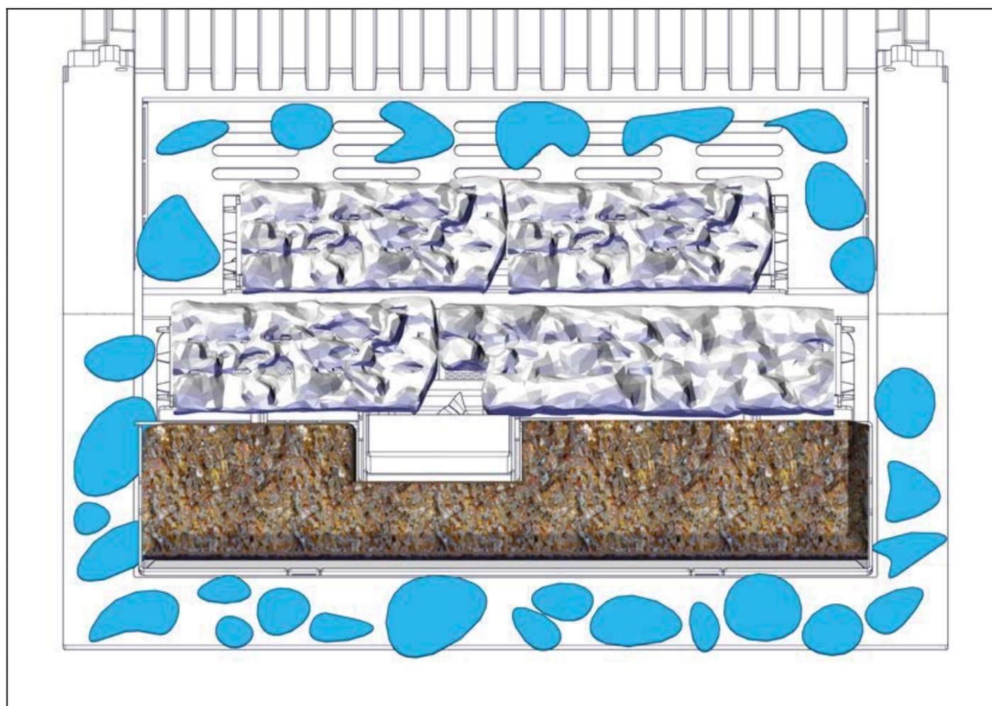
5. Put the charcoal pieces and chips of wood at the designated places around the burner bed. Refer to 2.6 for the numbers of the items.
