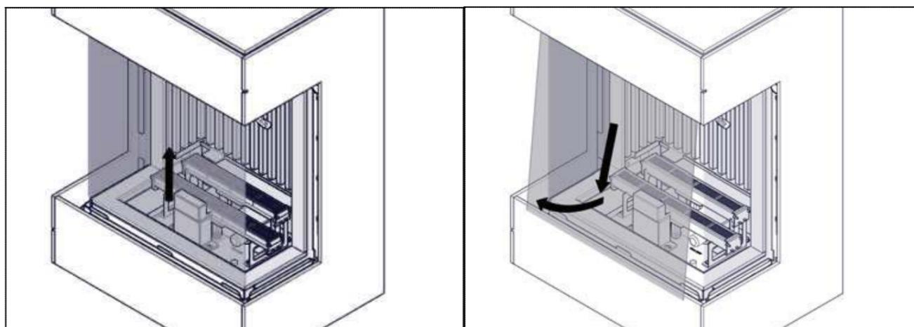
5. Loosen the screws left and right of the top side strips. Do not remove the screws and strips.
