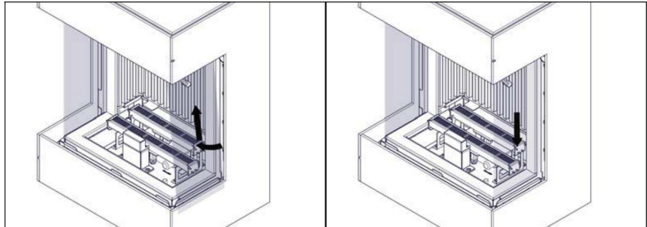
3. Tighten the screws left and right of the top side strips.
