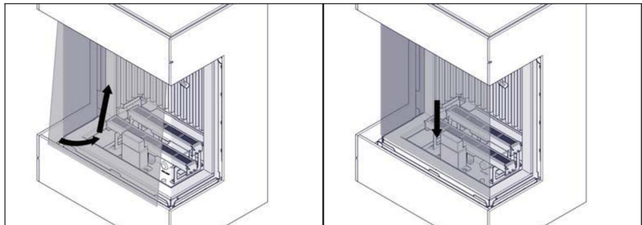
5. Lock the fastening levers on the top left and right of the glass panes.
