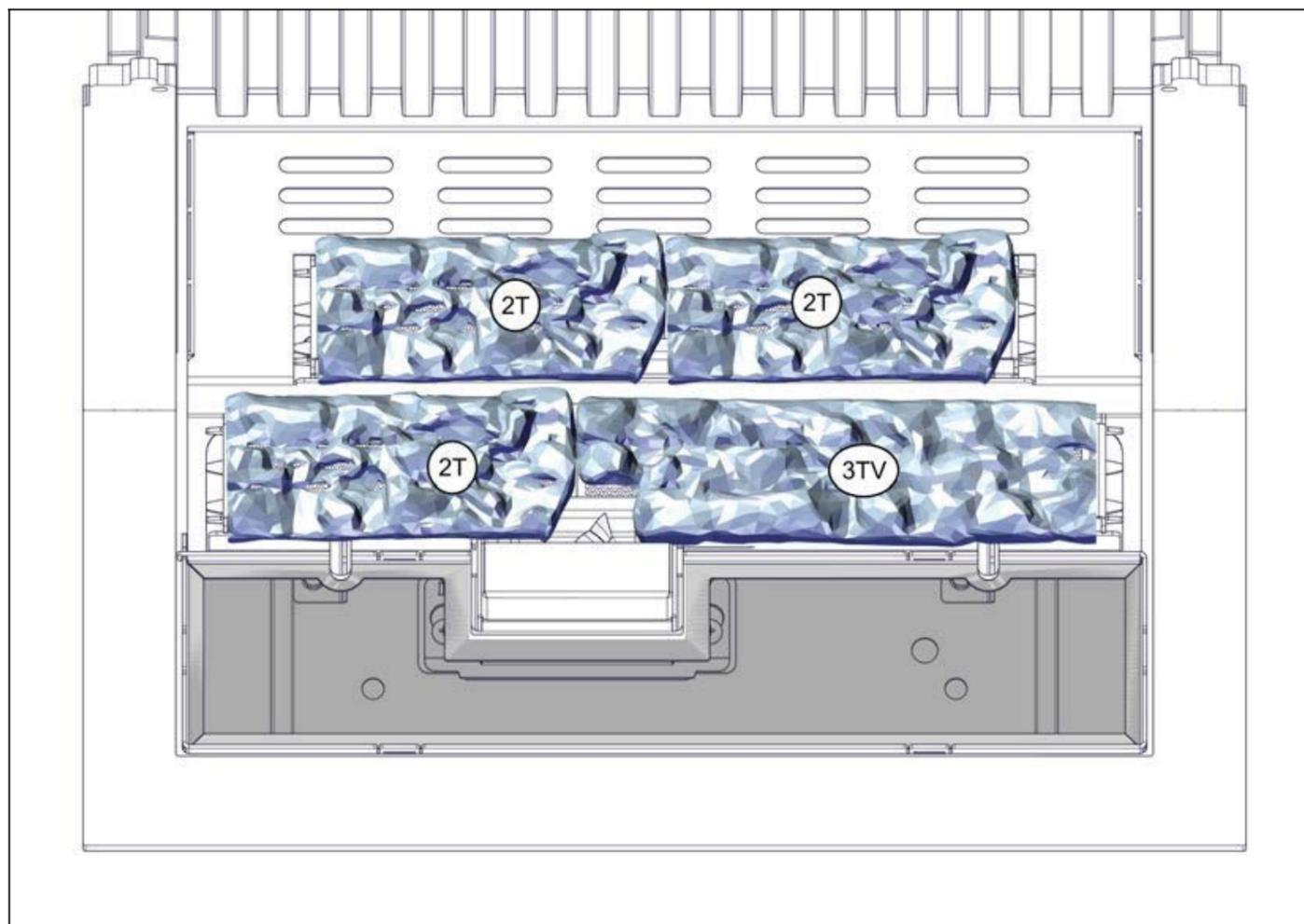
3. Spread the fire glass -dark amber- evenly on the metal grate in front of the burner bed.
