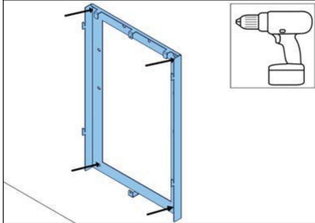
3. Attach the support frame to the wall with appropriate screws. Use plugs when necessary.
